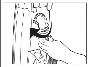
4. Twist the hose from the coupling elbow on the back of cleaner. Check for blockages at cleaner opening and in hose. If a blockage is found, clear the blockage.
